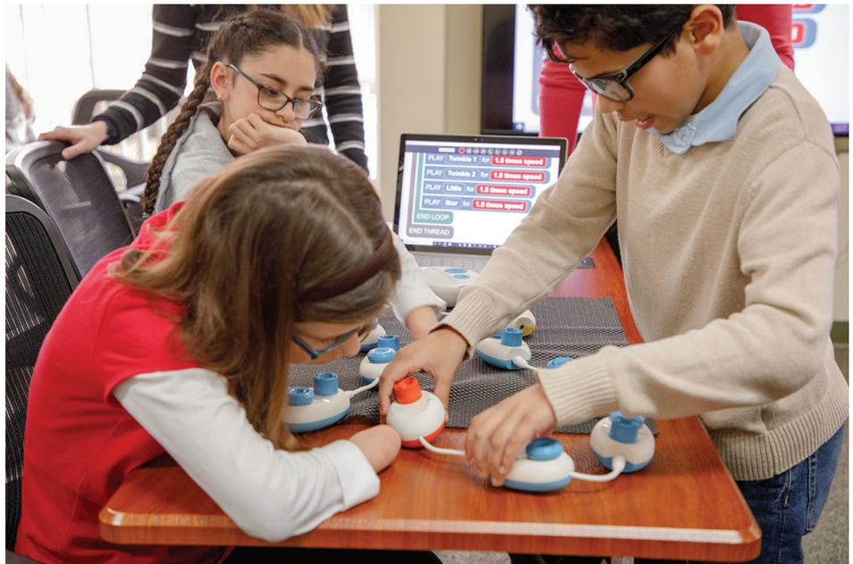
Code Jumper is made up of a series of small white pods, about the size of a potato, each with two dials of the same color on top and one thick white wire sticking out the side. Kids connect the pods with the wires and each pod represents a statement in a computer program.
